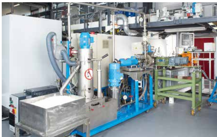
Fig. 2. View of the extrusion line: During pellet production it was important to optimize the quality by regulating water pressure, temperature and blowing agent content (© Fraunhofer ICT)
