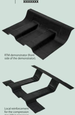
moulding processes, made from UD tape.
