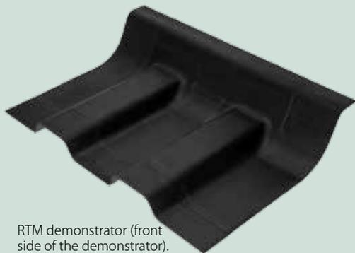
RTM demonstrator (front side of the demonstrator).
