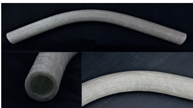
Fig. 2. Hollow profile formed by local stretch bending
