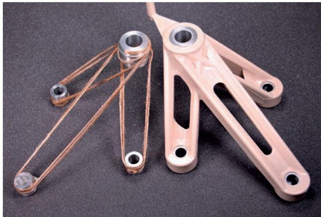
**Fig. 2.** Demonstrator of a three-dimensional structural component with metallic load application elements which allow applied loads to be transferred directly to the continuous fiber-reinforcement (© Fraunhofer ICT)
