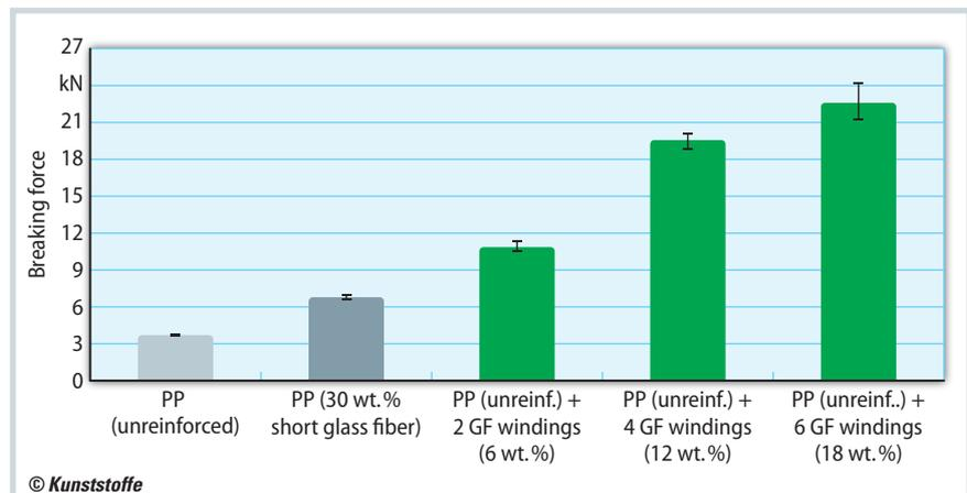
**Fig. 3.** Breaking forces of a simple pull loop with polypropylene (PP) depending on the number of windings. With six continuous fiber windings, the breaking load is already 500% higher (source: Fraunhofer ICT)
