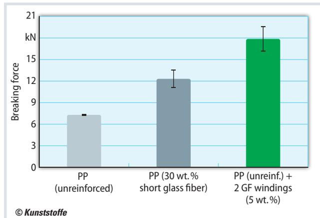
**Fig. 4.** Breaking loads of a generic 3D structural component with polypropylene (PP) can be significantly increased by wound continuous fiber-reinforcements (source: Fraunhofer ICT)
