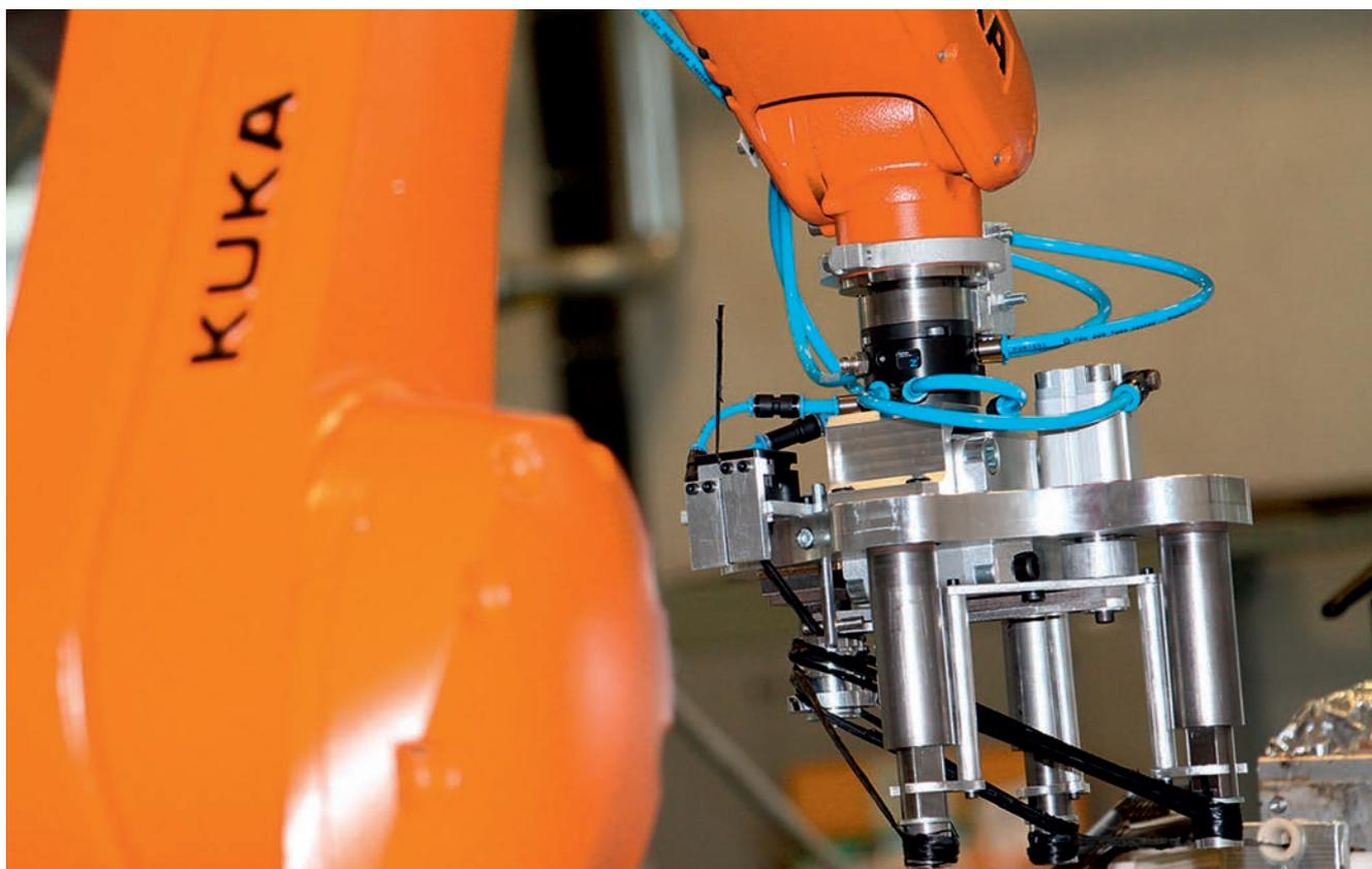
Robot-based fiber winding of complex injection molding inserts. The complex contours cannot easily be draped with flat reinforcing semi-finished products (© Fraunhofer ICT)
