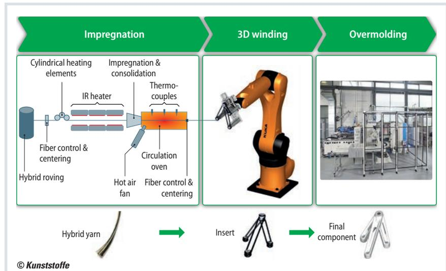
**Fig. 1.** The three-step process chain of the 3D skeleton winding technology. A 6-axis industrial robot places the molten hybrid yarn around the load application elements (source: Fraunhofer ICT)
