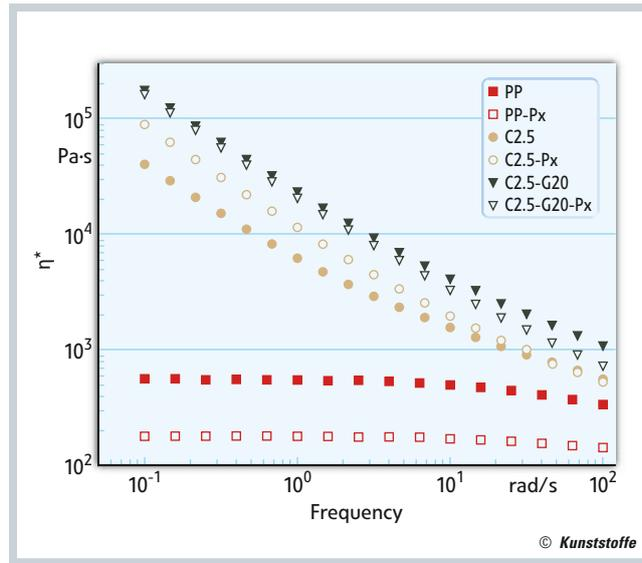
**Fig. 1. Complex viscosities of the tested materials** (figures: ICT)
