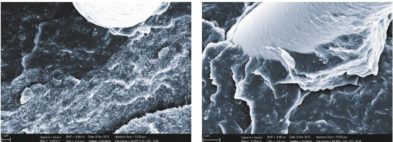
**Fig. 2. Typical morphology of the PP-CNT-GF composites without peroxide (left) and with peroxide (right)**
