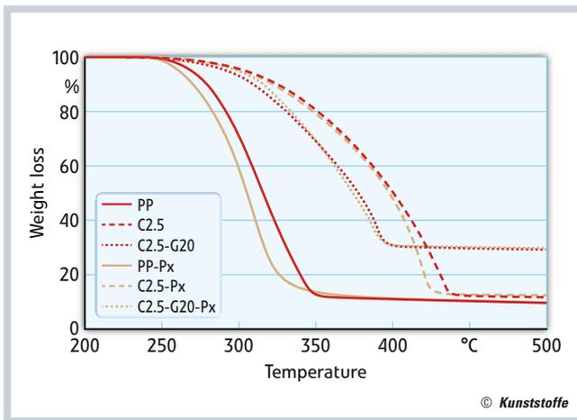
**Fig. 6. Thermal properties of the composites**
