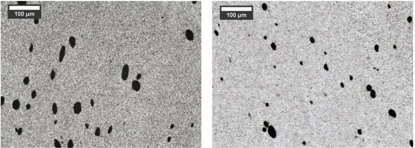
Fig. 3. Micrographs showing thin sections of the PP-CNT composites (2.5 % CNTs) without (left) and with (right) peroxide
