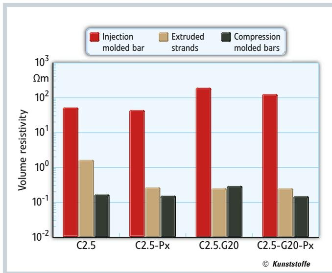
Fig. 4. Volume resistivities of the tested composites as a function of the method of processing
