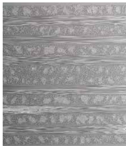
Fig. 2. Scanning electron micrographs (SEMs) of consolidated layups (cross-laminate) with low (left) and high pore content (right). The pores here are identifiable from the black and white areas (© Fraunhofer ICT)
