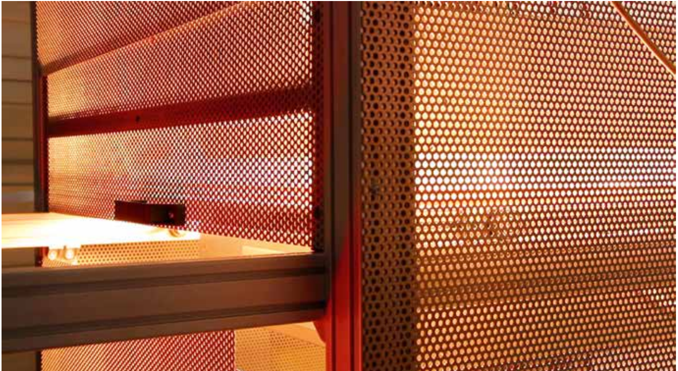
Heating module on the RVC line. The tape layup is heated with infrared radiation through the mold walls to a temperature above the melting temperature of the thermoplastic material (© Fraunhofer ICT)
