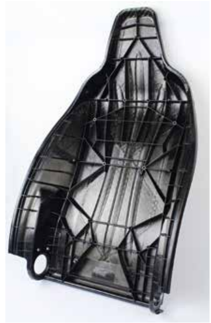
Fig. 1. Seat backrest demonstrator for process route 1 with molded-on reinforcing ribs and metallic inserts (© Fraunhofer ICT)
