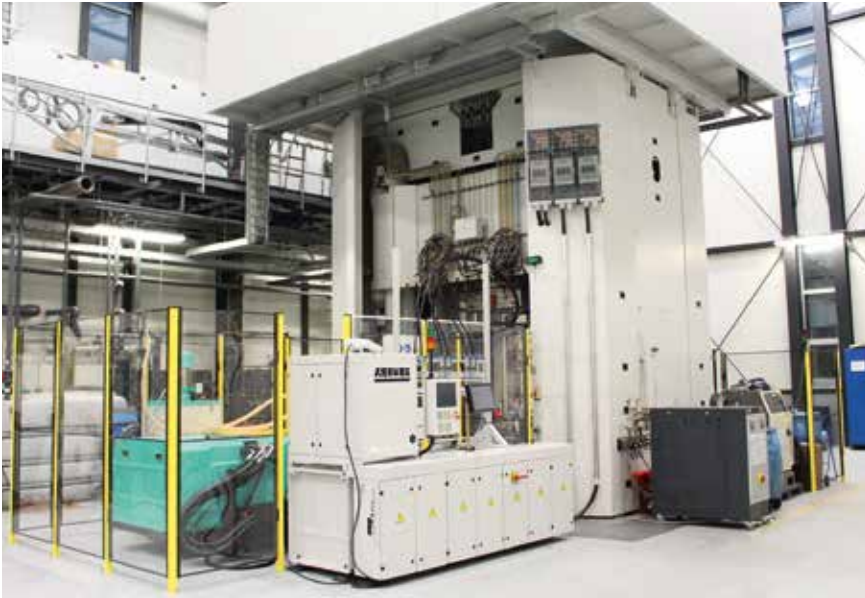
Fig. 3. Modular LFT injection molding module coupled with a hydraulic downstroke press for thermoforming and back-injection of laminated semi-finished products © Fraunhofer ICT
