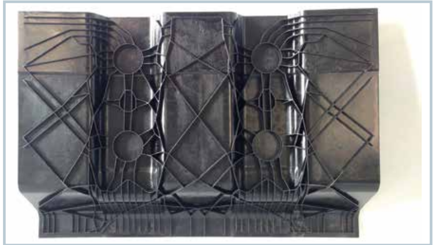
Fig. 4. Underbody segment of process route 2 with reinforcing ribs formed through extrusion compression molding (© Fraunhofer ICT)
