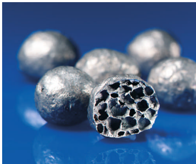
Fig. 2. The foamed aluminum particles (APM) are encapsulated with polymer foam (photo: Fraunhofer IFAM)
