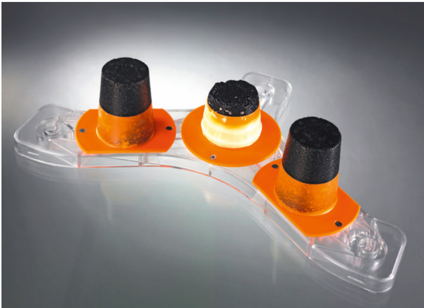
Fig. 4. The crash demonstrator consists of particulate EPP-APM hybrid foam bonded with an injection-molded semi-encapsulation
