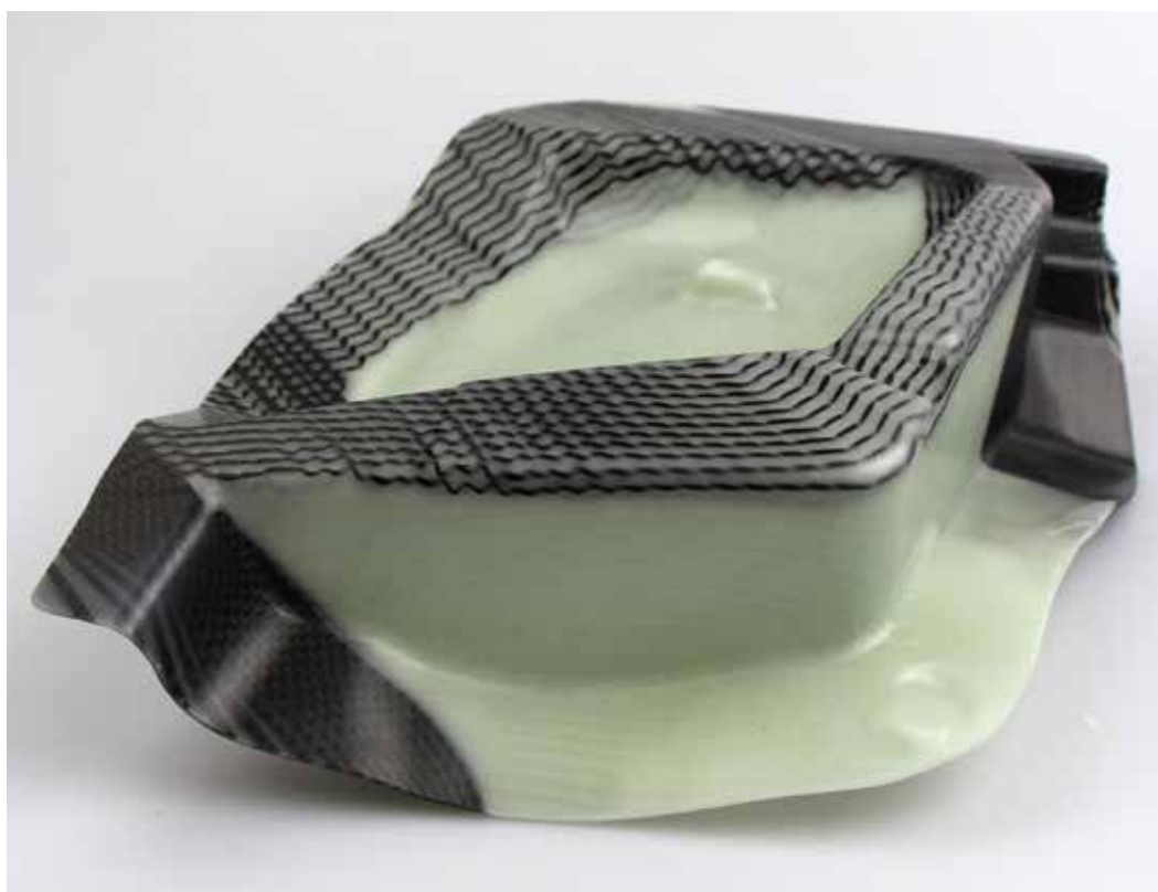
Glass-fiber-reinforced headlamp bowl with local carbon fiber reinforcement. It was possible to enhance the mechanical properties according to the load orientation through the multi-axial integration of carbon fibers into the basic glass fabric (© Fraunhofer ICT)
