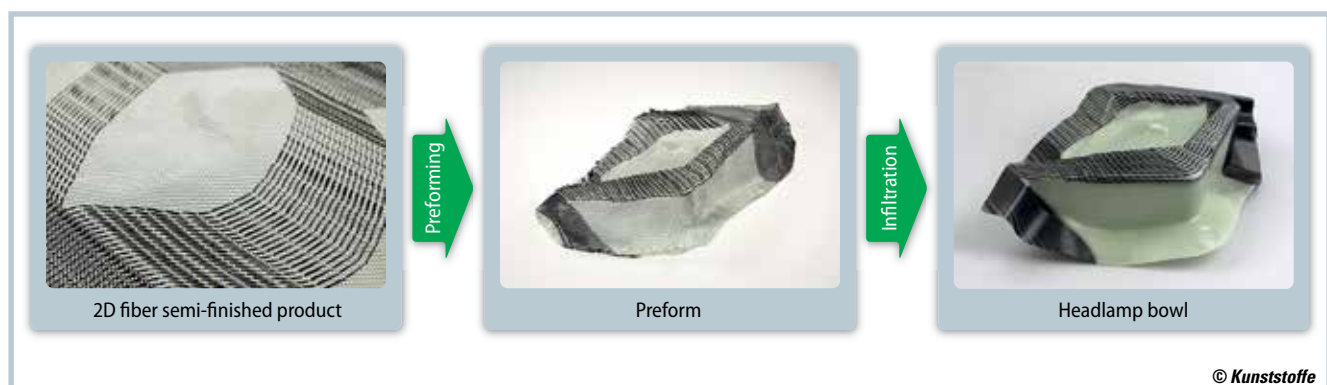
Fig. 5. Steps for the further processing of a fabric, which was reinforced multi-axially using ORW, to produce a finished fiber composite component: two-dimensional pre-cut fibers (left), fiber preform (center), infiltrated RTM component (right) (source: Fraunhofer ICT)
