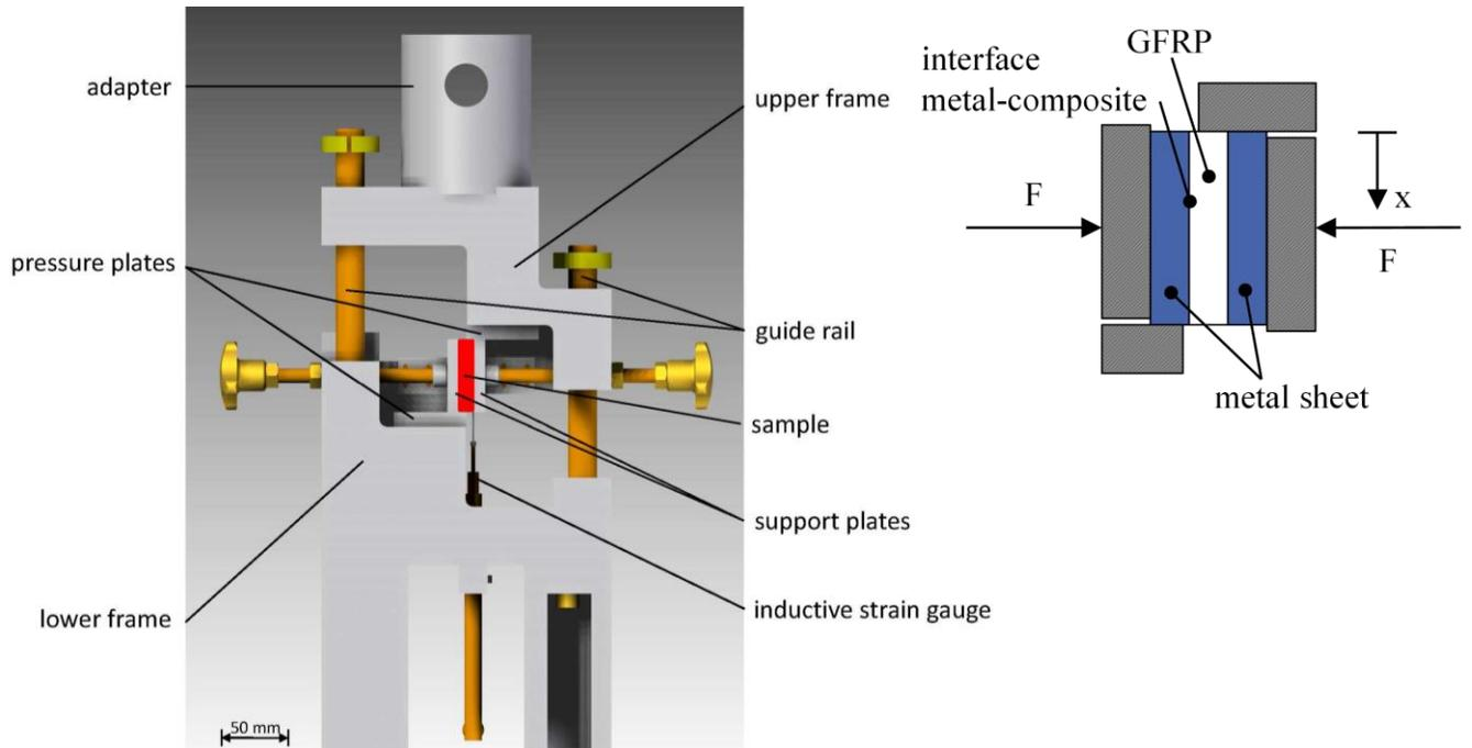
Figure 1: Schematic set-up of edge shear test rig [1] (left). Schematic detail view of shear plane (right).
