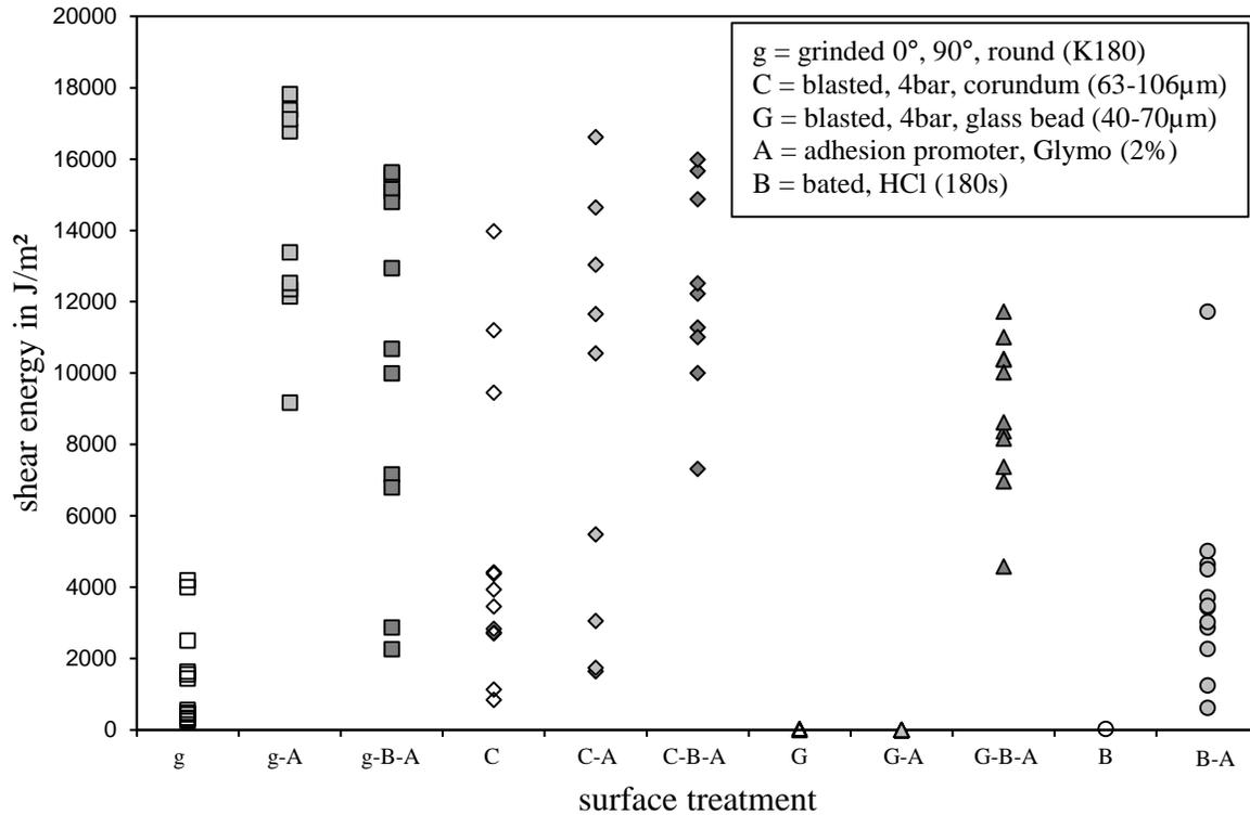
Figure 3: Diagram of shear energy.
