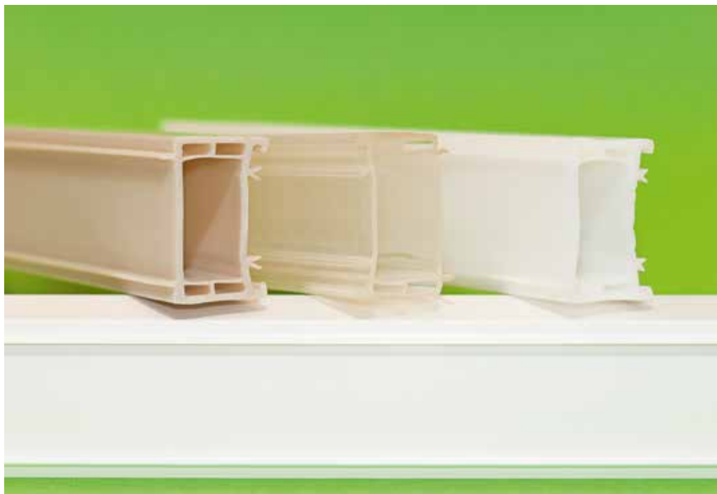
Profile made of polylactide (figures: ICT)
