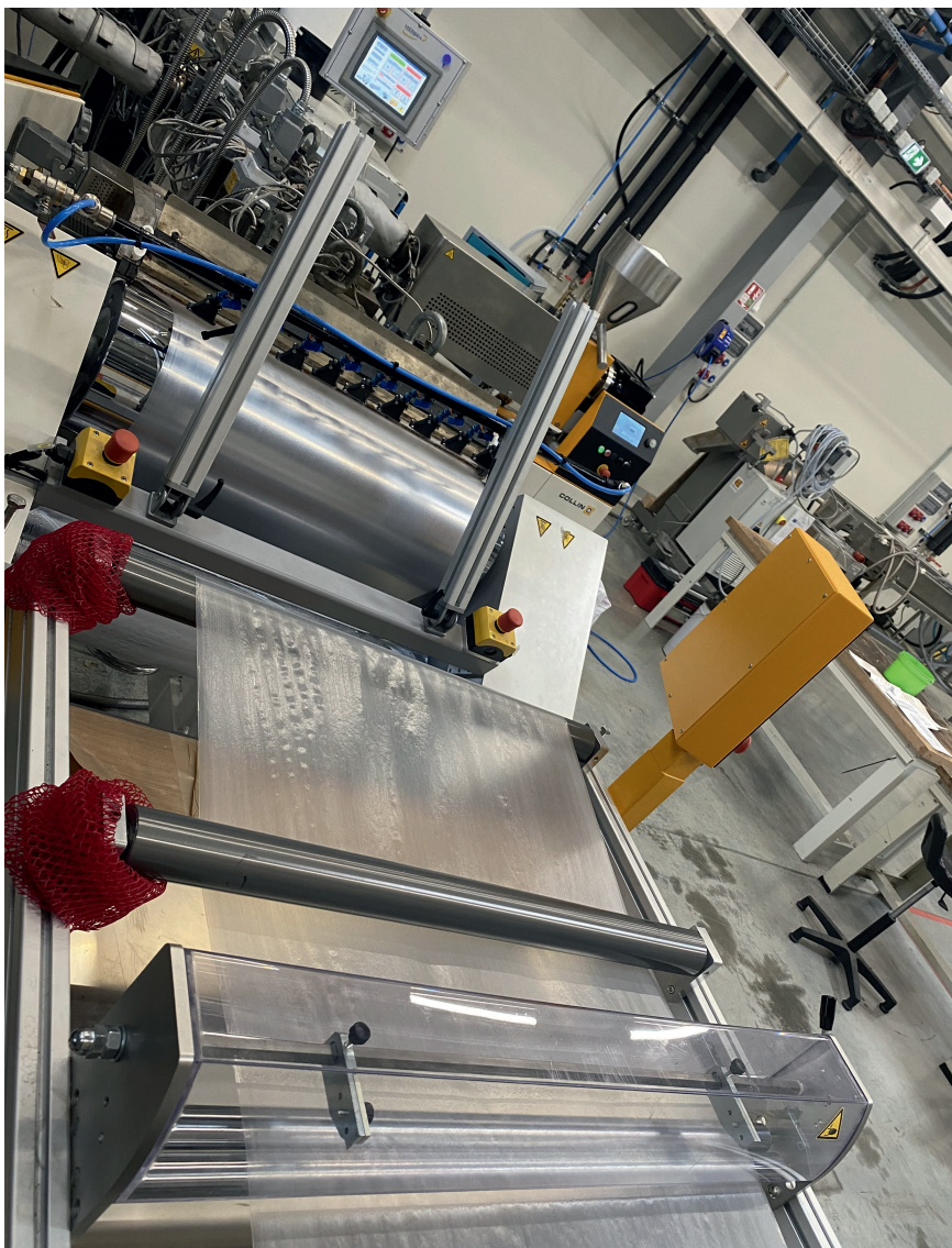
View into the IPC technical center: Production of the MultiNanoLayer film is running on the pilot line.
