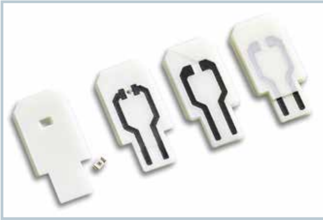
First, the black functionalized material with inserted LED, then the white ABS housing, is applied onto a build platform by an additive process (© Arburg)
