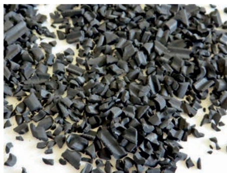
Fig. 1. Strings of production wastes (left) and shredded sprues of washing machine gaskets are fed back into the production of virgin material as fillers. © Fraunhofer ICT
