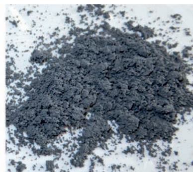
Fig. 1. Strings of production wastes (left) and shredded sprues of washing machine gaskets are fed back into the production of virgin material as fillers. © Fraunhofer ICT
