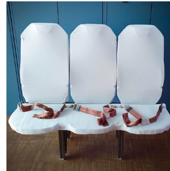
Fig. 5. The inner seat shell is manufactured using the WCM process. © Fraunhofer ICT
