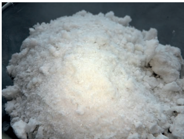
Fig. 4. Recycled bis(hydroxyethyl)terephthalate from the PET mixed fraction. © Fraunhofer ICT
