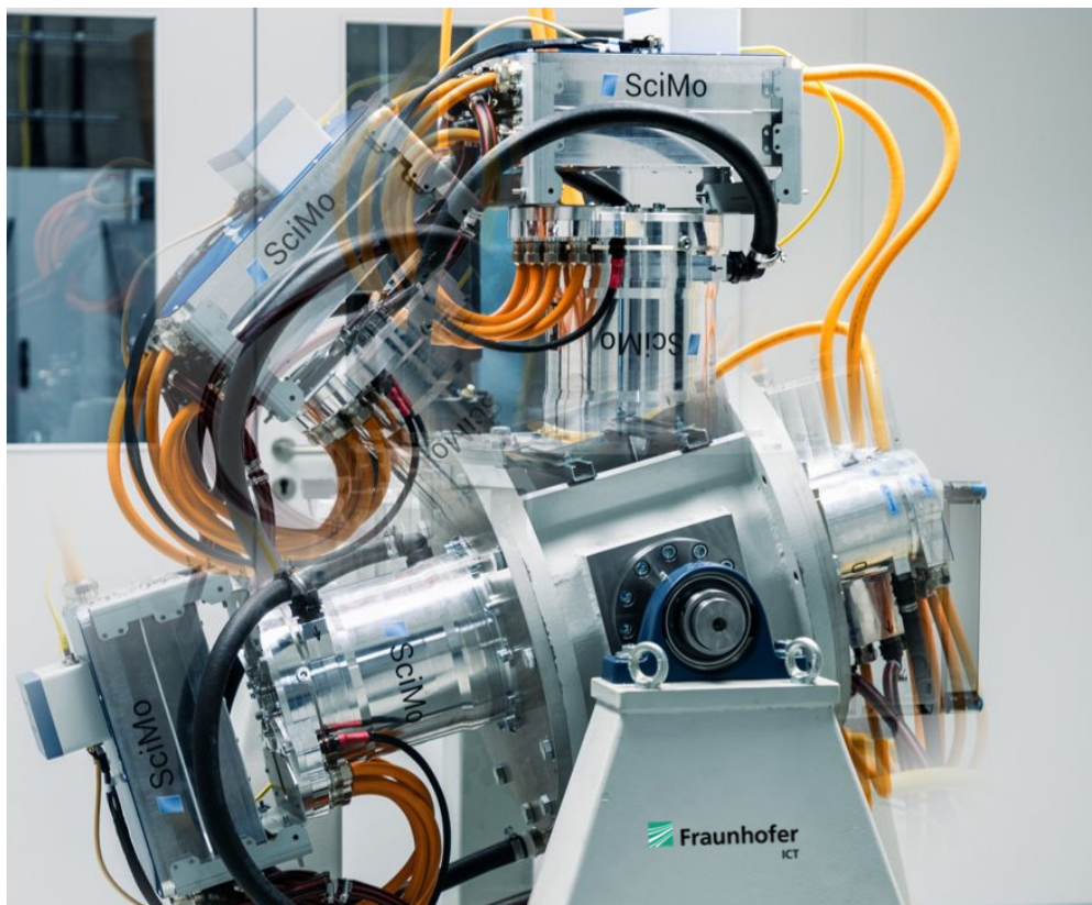
Swivel test rig for the validation of urban air mobility propulsion systems, © Fraunhofer ICT
