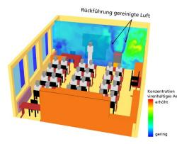
Numerical simulation of the aerosol dispersion within a classroom: An infected person sits in the front right corner of the classroom. The selected cross-section shows the concentration distribution of the virus-containing aerosol. A room air purifier filters the aerosol-laden air and returns it purified.
