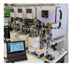
Device for the thermal inactivation of aerosol-borne viruses
