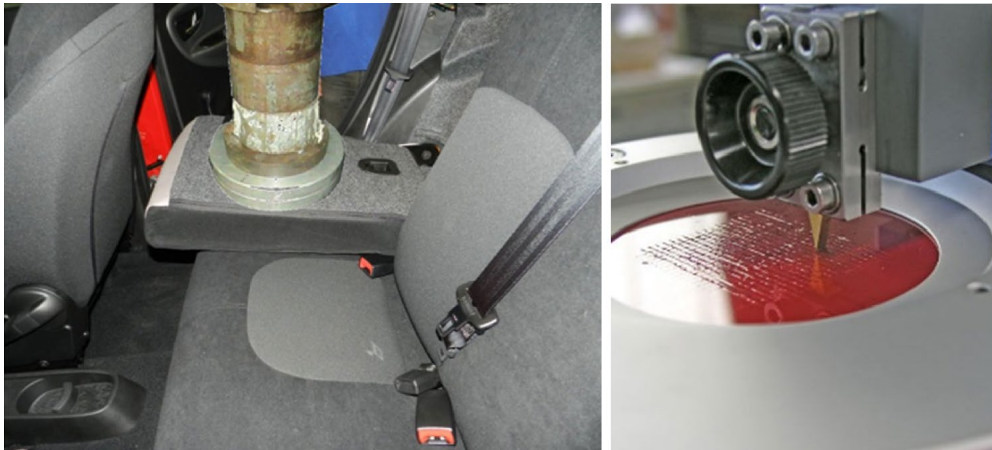
Figure 2. Experimental tests: overweight misuse (left), Erichsen scratch resistance (right)
