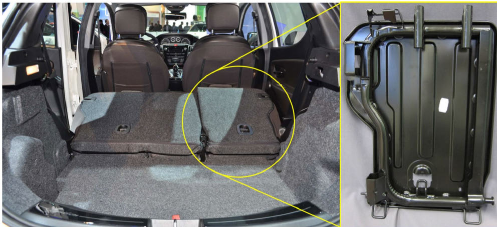
Figure 1. Current seat back, composed of a steel frame that supports a spot welded steel panel.
