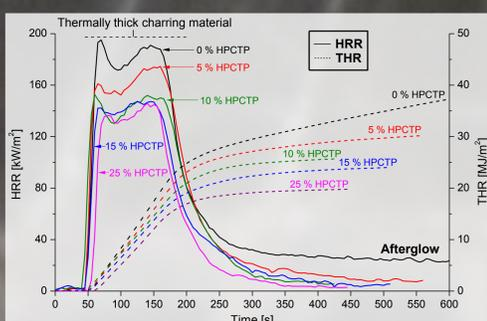
The Heat Release Rate (HRR) decreases with increasing HPCTP load. Without HPCTP, CFR APA6 shows afterglow. Incorporation of HPCTP eliminates afterglow and promotes char formation.
