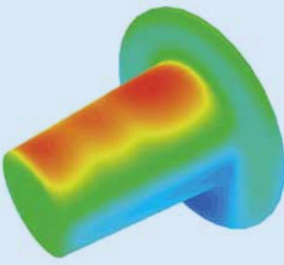
*Temperature distribution in a polymer component during solar simulation.*
