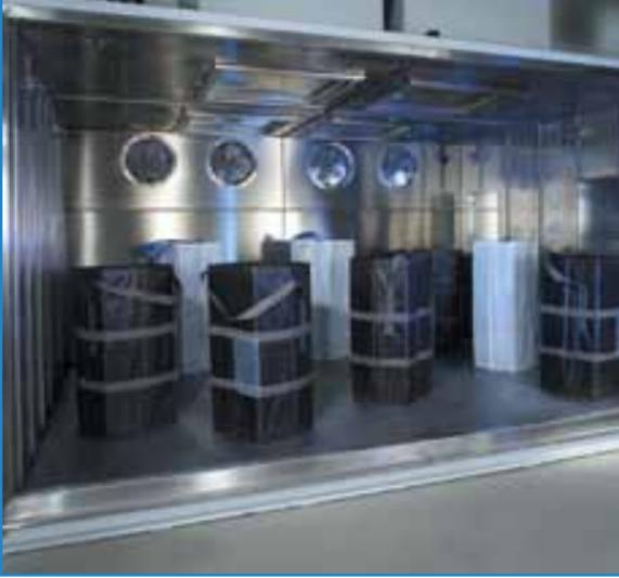
*Walk-in climate chamber (25 m<sup>3</sup>) with solar simulation.*
