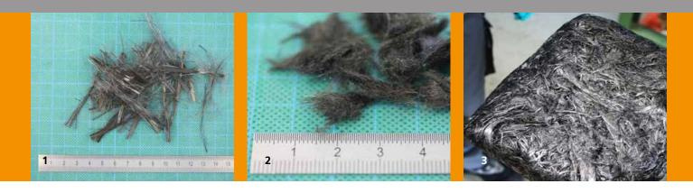
2 Fractions of shredded carbon fibers from the hammer and cutting mill.
