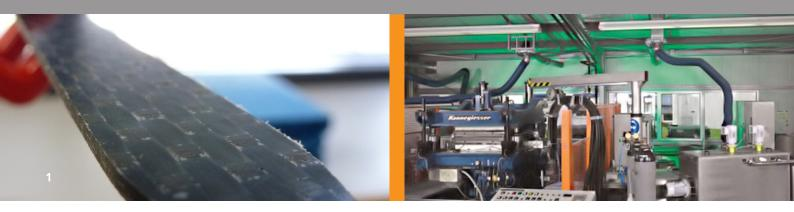
(Carbon fiber) reinforced cast PA6 (2 mm).
