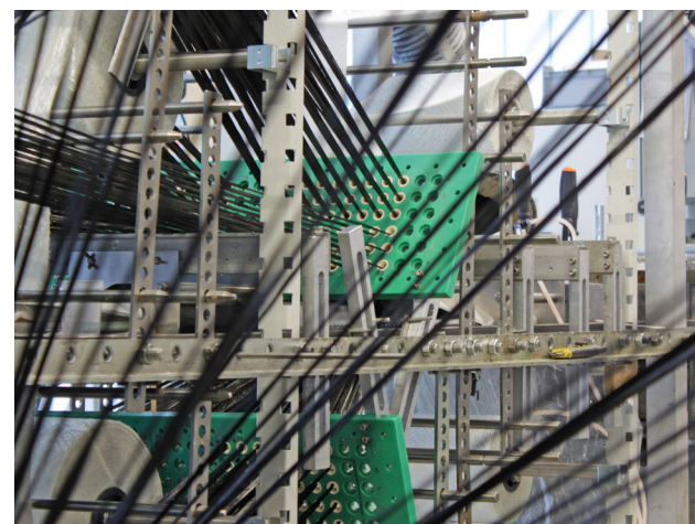
Pultrusion of a "Seat-Carrier" Profile
