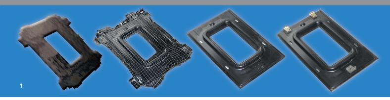
1 Process stages of a hybrid storage compartment flap made from thermoplastic UD tape (collaborative project involving the partners EDAG Engineering AG, Celanese – Engineered Materials and Fraunhofer ICT).
