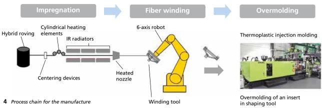
of thermoplastic winding components.
