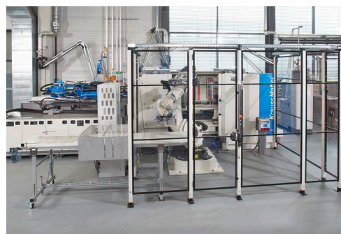
2 Fully automated injection molding machine to process granular thermoset molding compounds.
