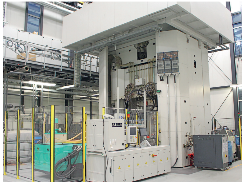
Combination of Arburg bold-on injection mold module and Dieffenbacher hydraulic press module
