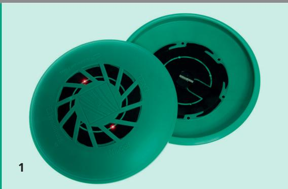
1 The demonstrator is a composition of molded plates made of electrically-conductive plastic, which are used for the power supply of two LEDs.
