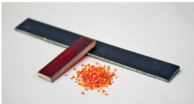
Virgin vitrimer based on disulfide bonds (left), ground vitrimer particles (middle) and recycled vitrimer via hot pressing (right).
