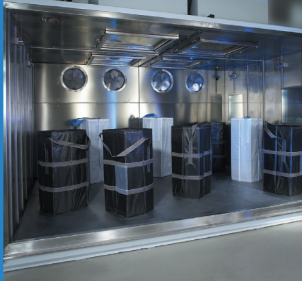
Walk-in climate chamber (25 m³) with solar simulation.
