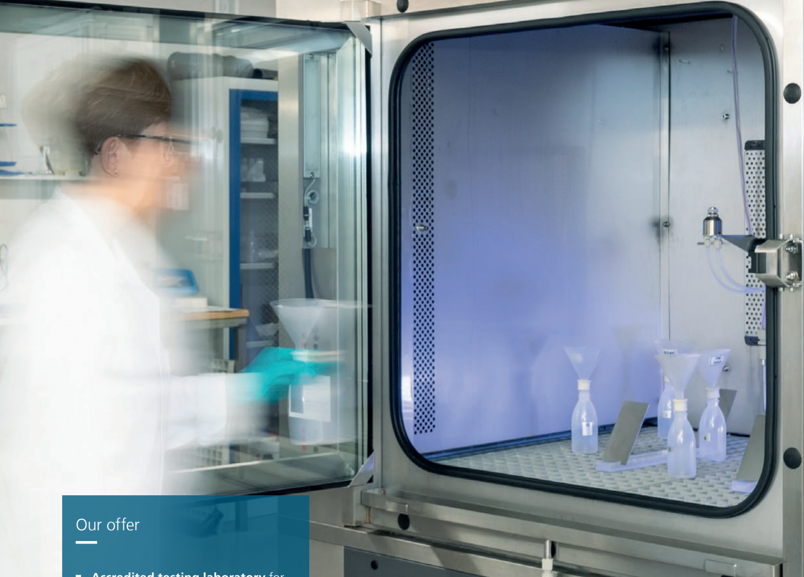
RSI FLCPLUS1000 corrosion test chamber with climate control unit
