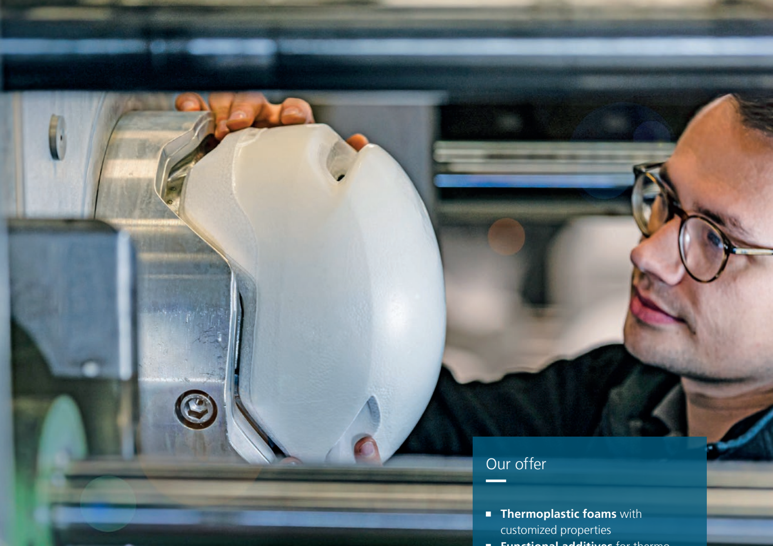
Production of a PLA helmet in an automatic molding machine.
