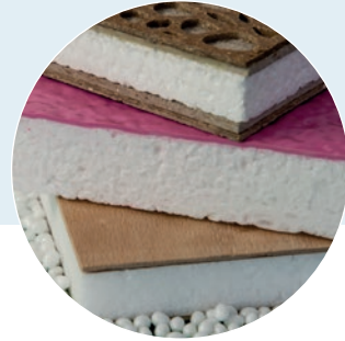
Sandwich structures with core foams made of renewable raw materials.
