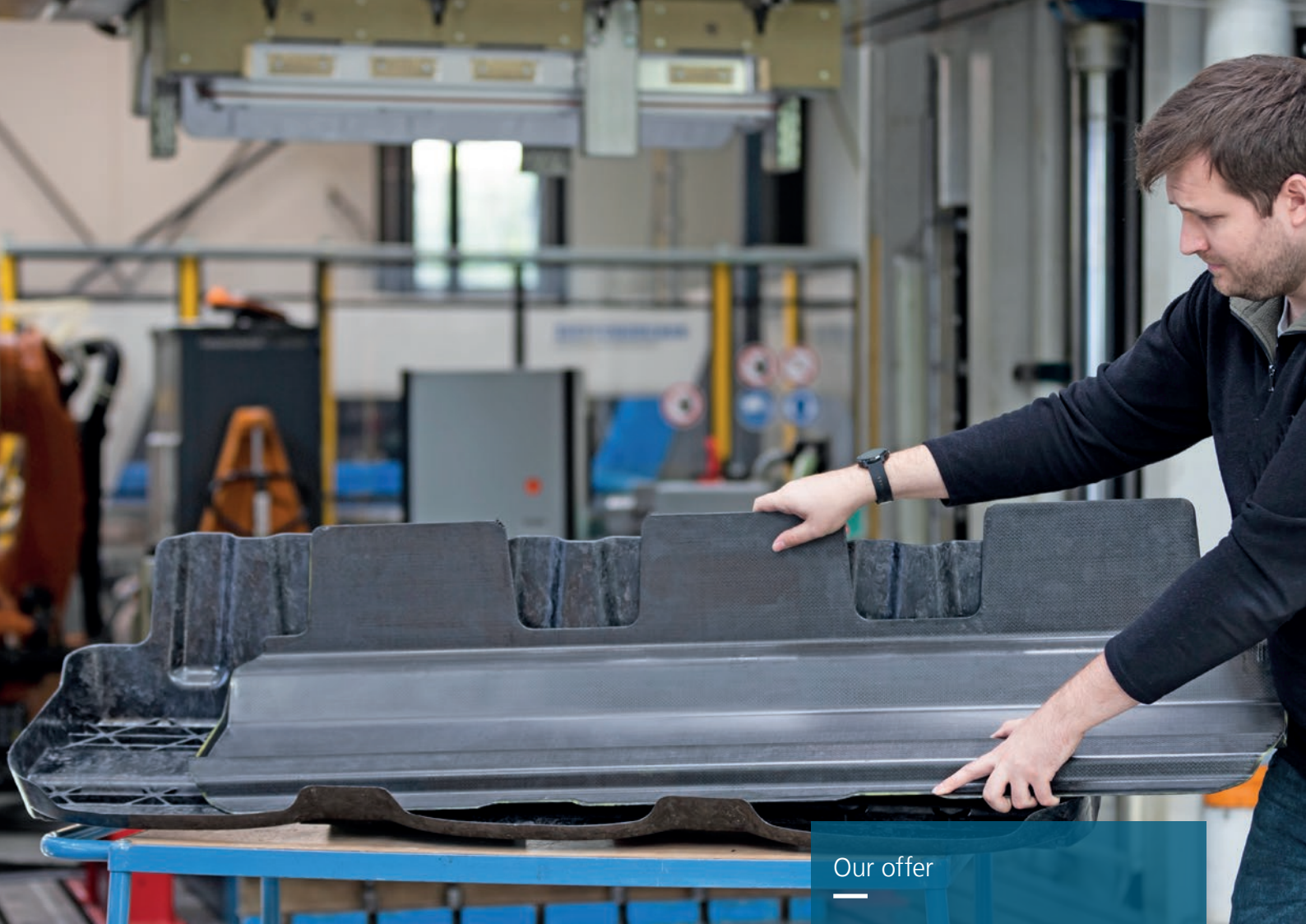
Seat shell made of carbon-fiber-reinforced SMC for commercial aircraft.
