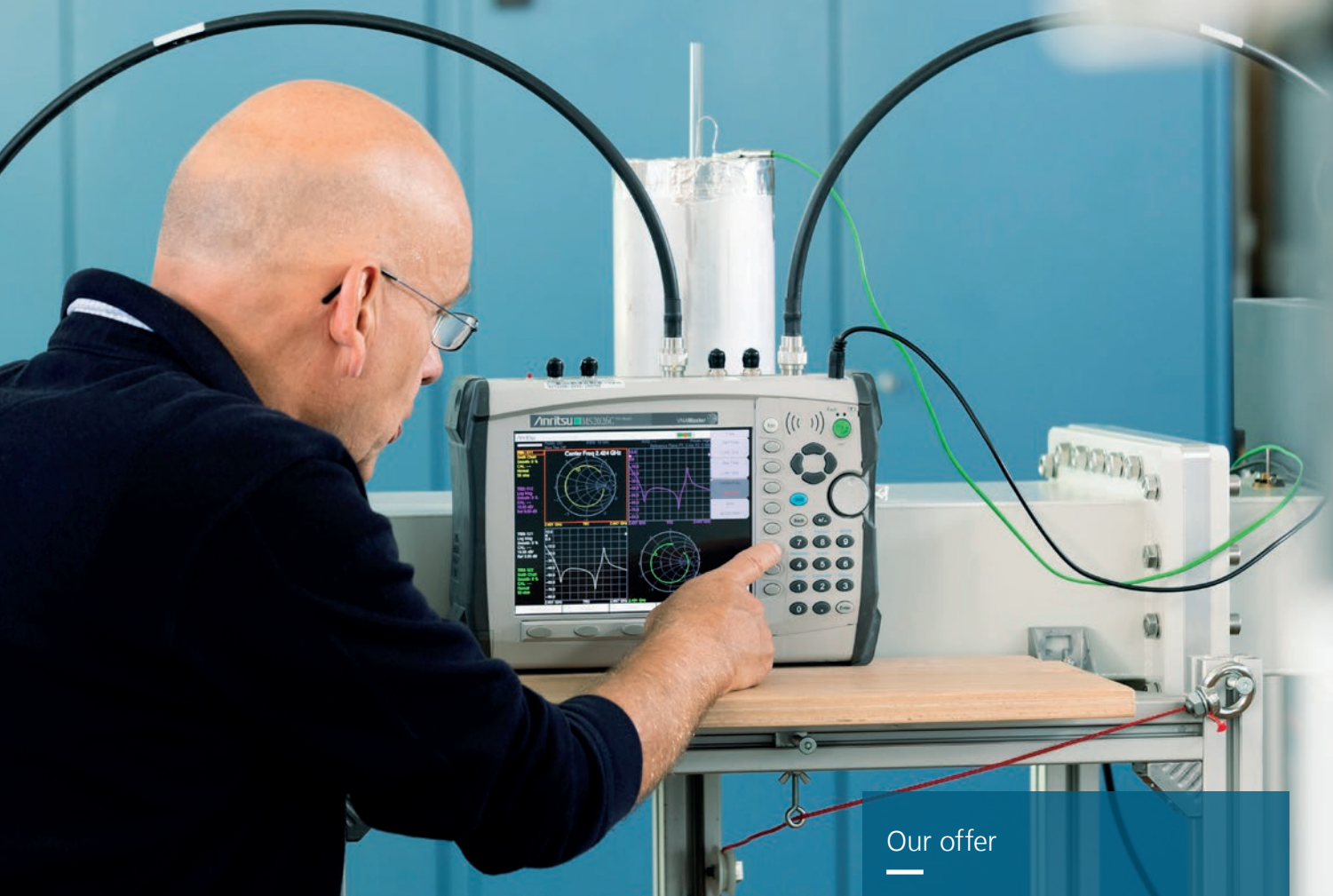
Apparatus to measure the permittivity of materials.
