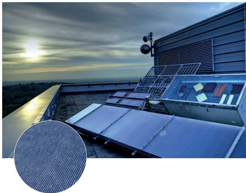
Natural irradiation and weathering of materials, e.g. sun and UV simulation.
