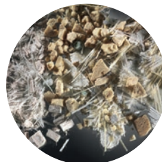
Shredded rotor blades as a starting material for high-quality fiber composite recycling.
