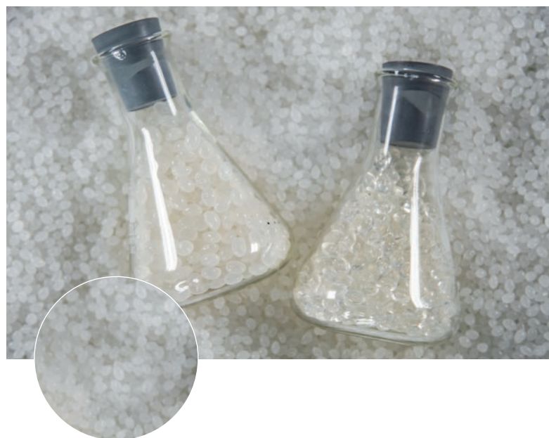
Poly lactide granules – the starting material for producing monomaterial systems.
