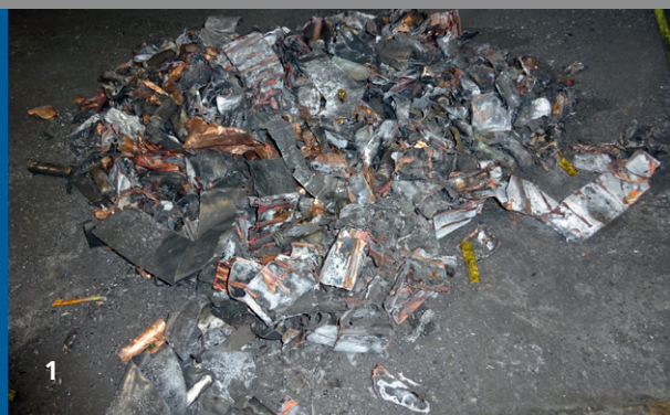
1 Cell residues after a safety test on a battery pack made of 18650 cells.
