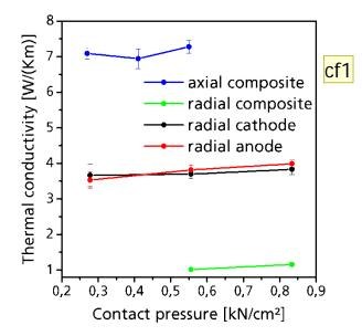
Thermal conductivity of cylindrical hybrid super-capacitors in axial and radial direction from the composite (cathode/ separator/ anode), and the radial conductivity of cathodes and anodes
