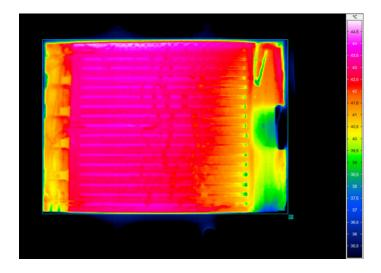
Thermograph of an air-cooled pouch cell for the verification of thermal simulations
