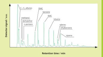
Time-resolved gas analysis exemplified by organic carbonates released after a cell shear test.
