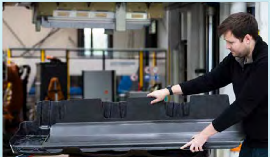
SMC (below) and WCM (above) component of the seat structure Photo: Fraunhofer ICT.
