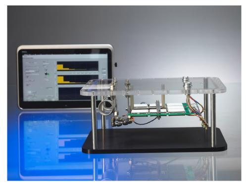
Temporally and locally-resolved reaction calorimetry in continuous reactors. The measurement software, which was developed on the basis of LabVIEW, enables the graphical visualization of the measured heat flows. (© Fraunhofer ICT) **PRESS RELEASE** June 7, 2018 || Page 2 | 3
