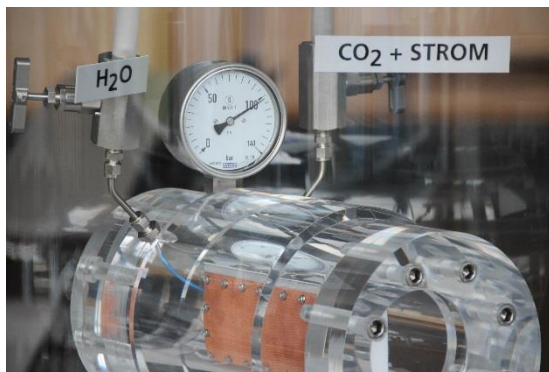
Image 2: Model of the high pressure electrolysis. (© Fraunhofer UMSICHT)
