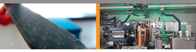
(Carbon fiber) reinforced cast PA6 (2 mm).
