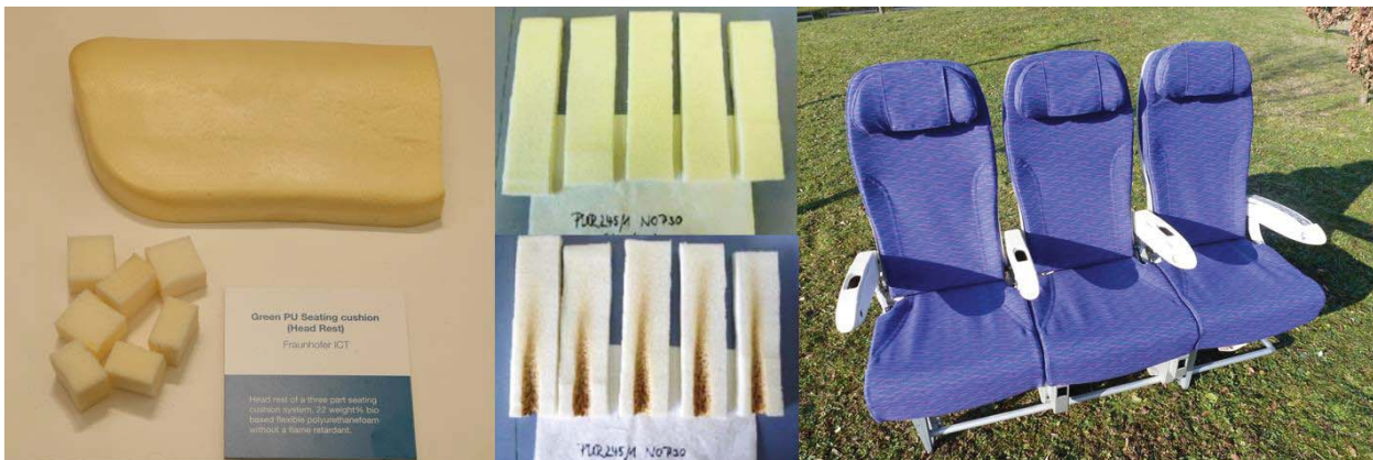
Figure 3: From left to right: Green PU seating cushion (Heat rest), Samples from Green PU foam before and after FAR 25.853 test, Aircraft seat bench with green PU seating cushion.
