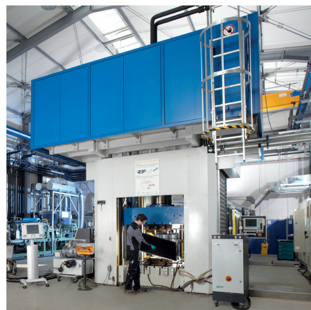
Schaumtandex extrusion line (left) and high-pressure RTM processing unit consisting of a hydraulic press and a high-pressure injection unit for the production of high-performance fiber composites (right).
