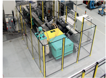
Modular long-fiber injection molding unit combined with a 3,600 ton press.
