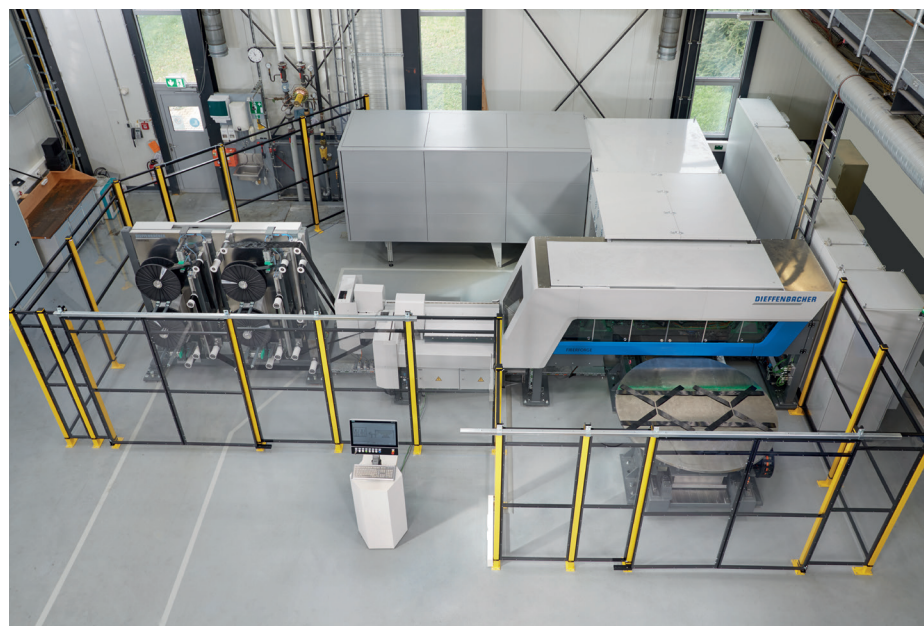
Injection molding production cell for processing free-flowing, thermoset materials and thermoplastic injection molding pellets (left) and Fiberforge system for fully automated processing of unidirectional fiber-reinforced thermoplastic tapes (UD tapes) (right).
