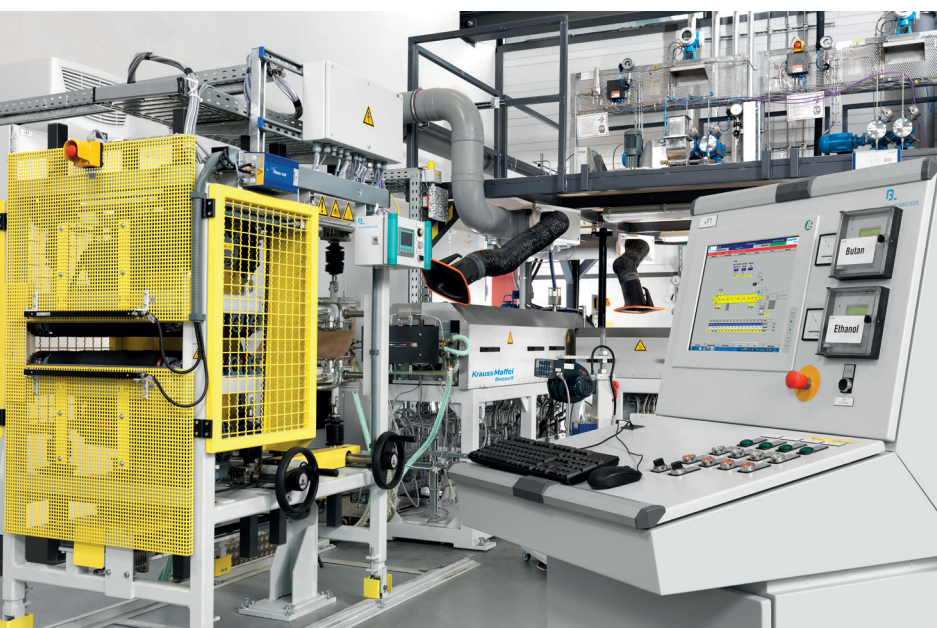
Schaumtandex extrusion line (left) and high-pressure RTM processing unit consisting of a hydraulic press and a high-pressure injection unit for the production of high-performance fiber composites (right).
